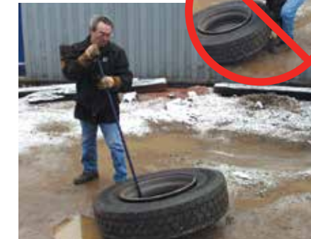
Specially designed forged knob end for hub side up
