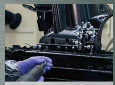
Can be rivet-bonded or weld-bonded immediately after application
