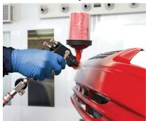
With the new 1.2 mm and 1.3 mm atomizing heads, you can go from start to finish on bumpers: primer, sealer, basecoat and clearcoat.
