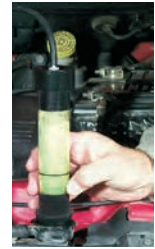
LEAK DETECTED (FLUID CHANGES TO YELLOW COLOR)
