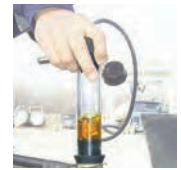
LEAK DETECTED (FLUID CHANGES TO YELLOW COLOR)
