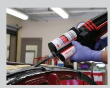
May be used for bonding door skins, quarter panels, roof skins, box sides, van/ utility vehicle sides and rocker panels when recommended by OEMs.
