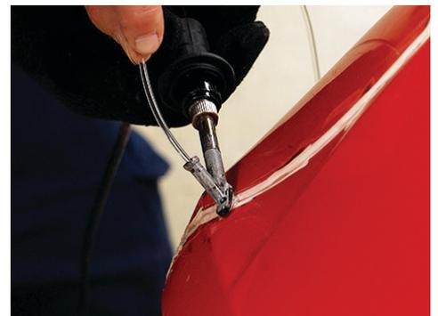
Use the airless welder to smooth hot air welds or to repair thermoset polyurethane (PUR) bumpers and truck bedsides with included welding rod.
