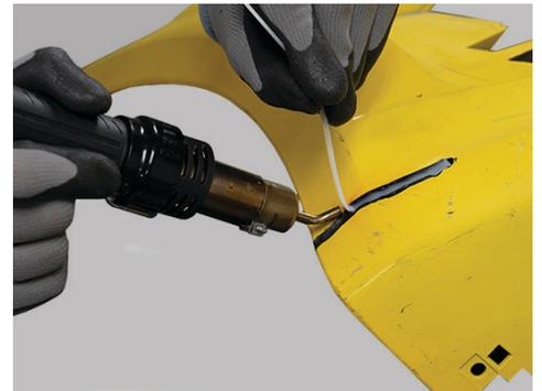
Use the hot air welder to make fast, strong welds on thermoplastics with included ribbon rods.
