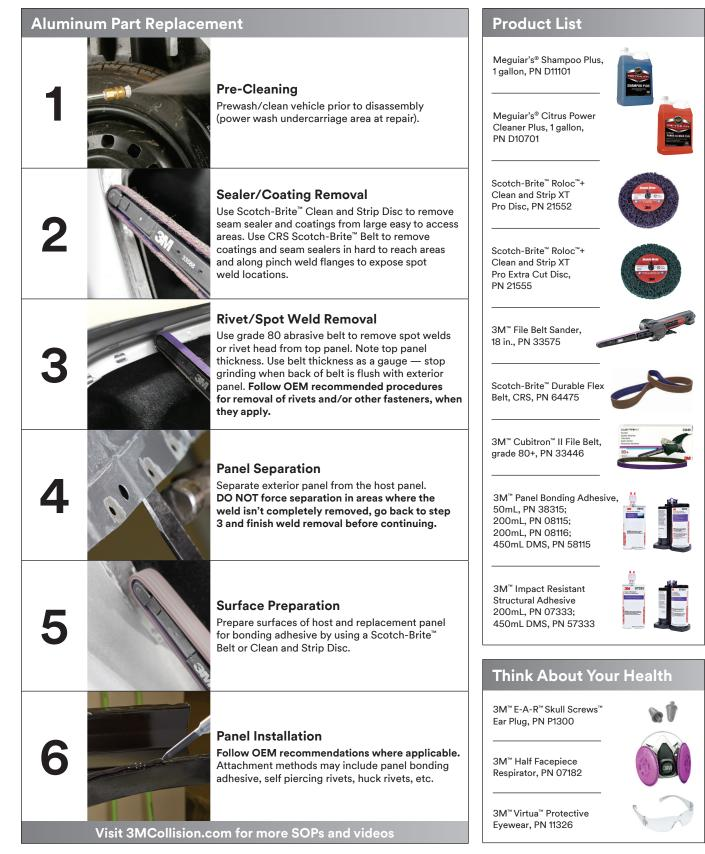
Note: Use caution when working on aluminum parts. Use tools that have been cleaned properly or designated for use on aluminum to reduce potential cross contamination. Do not re-use abrasives that were previously used on steel repairs.
