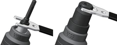
Install a new mandrel and nosepiece to match your intended rivet nut thread size. Use the included wrench to install the new mandrel into the #2 Plunger Tube. Ensure that the mandrel and other components are tightly fixed in position. After installing the front bushing cover and lock bushing, lightly tighten the new nosepiece onto the end of the tool. Install the hex shank drive end of the tool into your drill and affix tightly into its chuck.
