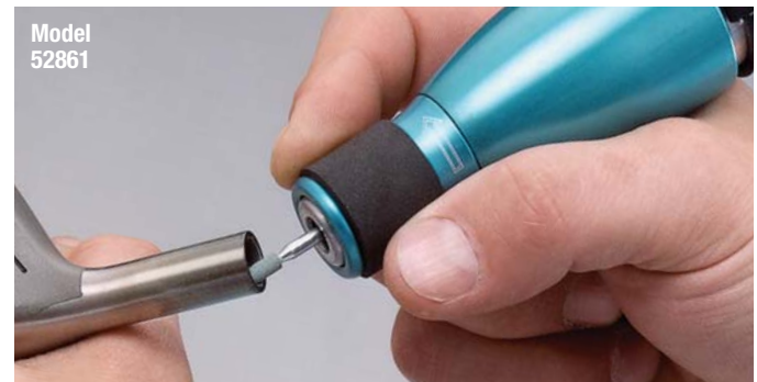
Rotary Vane Pencil Grinder is ideal for precision deburring.
