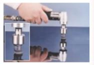
Excellent for removing dust nibs on clear coat paint systems using various sanding heads and sanding pads.
