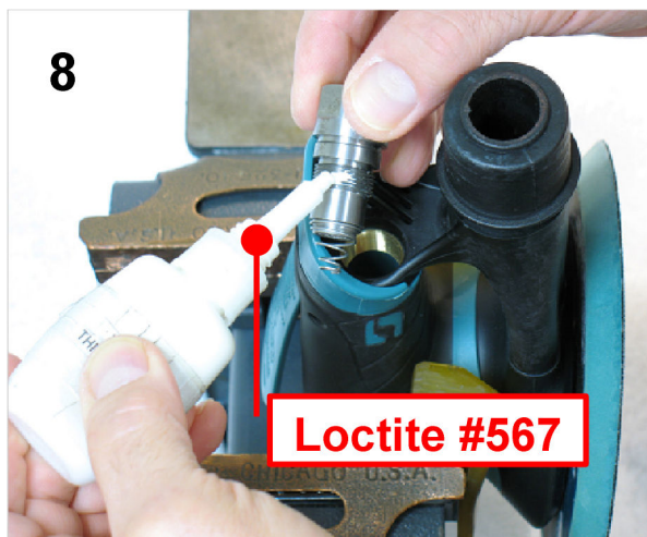
Apply a small amount of Loctite #567 to 59335 Inlet Bushing.
