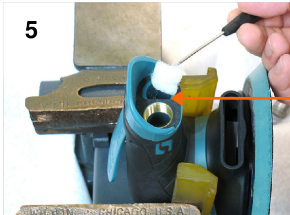
Remove 56027 Muffer Inserts (5). Disassembly completed.
