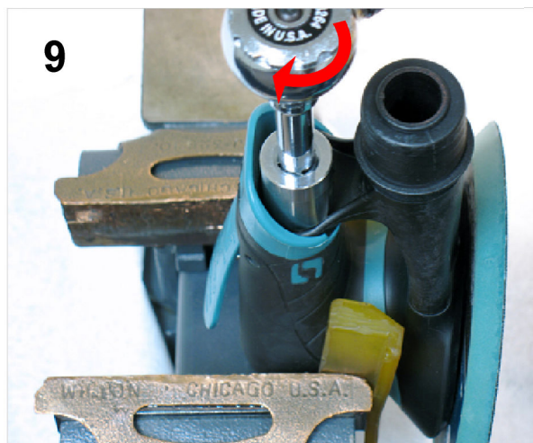
Install 59335 Inlet Bushing. (Torque to 23 N·m/~200 lbs. in. )
