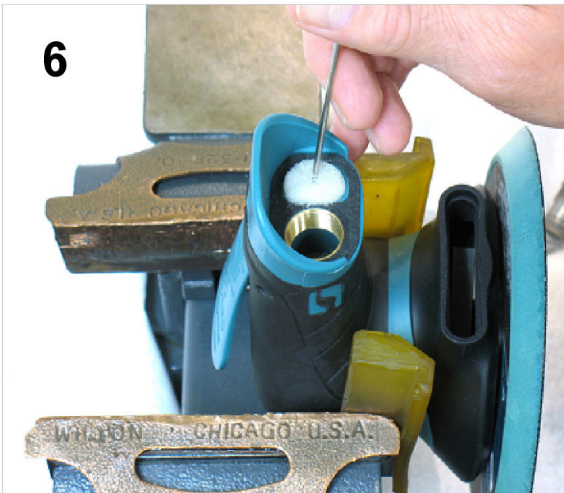
Install new 56027 Muffer Inserts (5).
