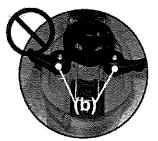
Incorrect locking of cams (b) could result in leaking and/or the lid detaching from the can.
