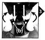
To lock the locking cams (b), push and turn cams towards the inside.
