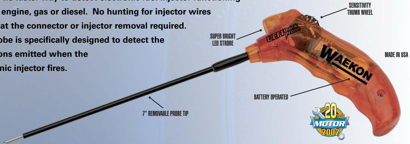
Simply press the 7" long probe tip against the injector body, adjust the sensitivity using the thumb-wheel and the bright LED strobe will flash each time the injector opens and closes. The strobe allows the you to determine if the injector is firing consistently, misfiring or not firing at all.
