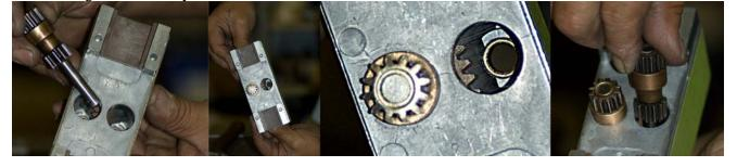
3.Place the top gear 1227 by the gears. Use an arbor press to press both 1209 & 12010-1 flat. Press one at a time. The extra gear will let you know when to stop.
