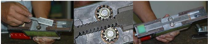
12. Placing the 1204 drive shoe is just the opposite. This part is lined up with gears, all the way to the front.
