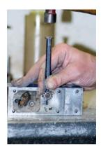
Use a 1/8 drift punch to push the 1252 pin out of the 1227 gear. Push pin out just enough to free 1210-1 gear
