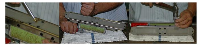
14. Install Hutchins pad, always put the whole on top towards the rear of tool. Run the tool flat on the bench, under a full person's weight. You should not be able to stop the tool. Never use 3M pads! These will bind on the bottom of the tool, and cause extensive damage.
