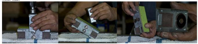
5.Use Spray gasket glue or Silicone Sealant on 1214 Valve Plate. When tacky, place on motor block with 1225 timing plate towards front.
