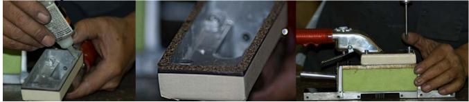
10.Clean any excess glue off. Turn over tool and check gears to make sure they spin freely. Prepare to install 1242 counterweight bar. Install 4-1207S ware strips. Press in with holes towards center gears. Glue
