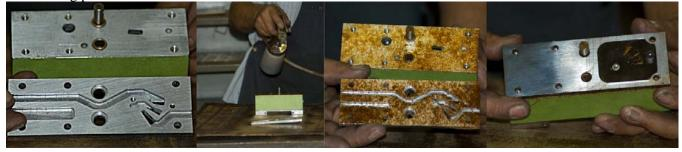
6.Use new 1212S gaskets and glue onto each end of motor block. Make sure to put gasket on, so airway is not blocked. The center hole has a notch. Align that towards the top of the tool. Attach 1217 front with screws, and small clear washers. Hand tighten screws, then tighten with screw gun. The 1218 rear can then be attached in the flowing order: 1220 gasket, 1218 rear, 1222 gasket, & 1223 muffler. Screws with no washers are used.
