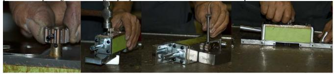
8.Prepare 1228S. Place puck inside sector opening then add washer & screw. Place on top of housing lining up the last tooth to the right. Test turning the sector to make sure you have the correct tooth. When turning back & forth, the sector set should not go over the edge of the block. Turn 1228s to align in direct center,
