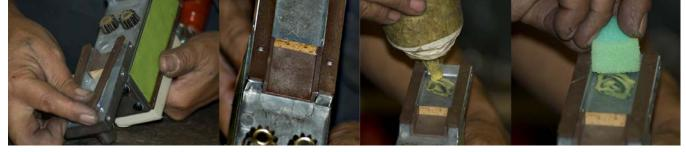
11.Hold tool in hand angling handle towards you body. Turn Right gear (1210-1 long gear) all the way counterclockwise till it stops. Put counterweight bar 1242 in, lining up spring first. The second tooth on counterweight bar will line up towards record feed.
