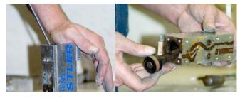
Pry off the 1214 Valve plate. The 1211 Piston and 1212S Piston Rings with ends will now come out. Rings should have no wear, and have a good seal. It is usually a good idea to replace these with each repair, unless the tool is very new.
