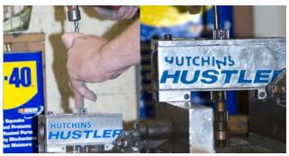
Place the 1215 Block on top of the two aluminum blocks. With a hammer and bit, tap out the 1209 and 1210-1 gears through the top of the valve plate. They should drop through the bottom of the block.
