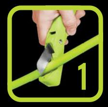
**CUT** – Remove damaged portion of hose or measure and cut desired length at 90° angle.
