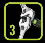
**TIGHTEN** – Tighten fitting nut until snug. Slide bend restrictor up and snap onto nut.
