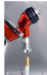
Placing Spray Gun on Nozzle Extension
