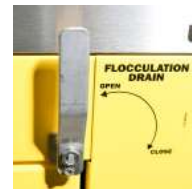
Flocculant Drain Valve
