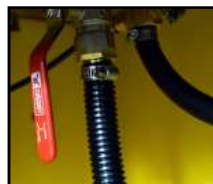
DRAIN VALVE - OPEN POSITION (HANDLE IN VERTICAL POSITION).
