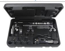
Includes heavy duty tube cutter 70033 for 1/8 to 1 1/8" 0.D. tubing; standard  $45^{\circ}$  flaring tool 70051 flares 7 sizes: 3/16, 1/4, 5/16, 3/8, 7/16, 1/2 and 5/8" 0.D. tubing; five double flaring adapters 70192 cover 3/16, 1/4, 5/16, 3/8 and 1/2" 0.D. tubing.
