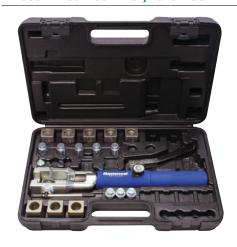
Fabricates "production quality" flares quickly and easily with hand held convenience. Flaring die sets for five sizes: 3/16, 1/4, 5/16, 3/8 and 1/2" 0.D. tubing; five double flaring adapters cover 3/16, 1/4, 5/16, 3/8 and 1/2" 0.D. tubing. Set includes:
