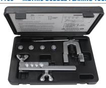
Fashions International Standards Organization (I.S.O.) bubble flare found on European, Japanese and some domestic model brake lines. Flares without removing brake lines from a vehicle. Includes hardened steel bar and carrying case. Set includes: Adapters for 4.75, 6, 8 and 10mm 0.D. tubing.
