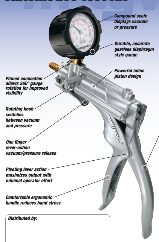
The new Mityvac **Silverline Elite hand** pump combines 35 years of automotive diagnostic experience with advanced performance and comfort to meet the requirements of the latest automotive technologies. Featured in the new MV8500\* **Silverline Elite Automotive Test Kit, the** pump produces vacuum along with pressure at twice its previous output to expand its vehicle service applications.
