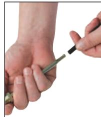
**1** Attach nylon tube to fitting.
