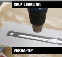
Use Self Leveling Seam Sealer or High-Build Self Leveling Seam Sealer for applications where a flowable sealer is needed.
