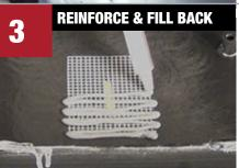
Mask front side of repair to prevent repair material from flowing through. Apply **Plastic Repair Contouring Tape** (mesh only) to back side. Apply **Dual-Mix**<sup>TM</sup> **Multi-Plastic Repair Material** or **Dual-Mix Problem Plastic Repair Material** and cover mesh tape. Spread material firmly. Allow to set.
