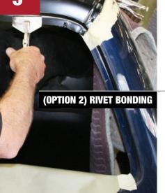
Clamp panel in place. Do not over clamp. Install rivets or STRSW per manufacturer's recommendations during adhesive's working time. Remove clamps after rivets or spot welds have been installed on panels fully supported by these methods. Wipe away excess material.
