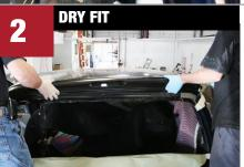
Dry fit all panels to ensure proper alignment. Drill holes or mark locations for:
