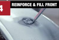
Remove tape from front. Fill front with **Dual-Mix Multi-Plastic Repair Material** or **Dual-Mix Problem Plastic Repair Material**. Spread material firmly and build up higher than panel to allow for sanding.
