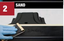
Sand primer with P180 grit. Sand bare metal with P80 grit. Blow off and tack clean. Re-clean with SEM Solve or XXX Universal Surface Cleaner. Wipe clean in one direction with clean, lint-free cloth.
