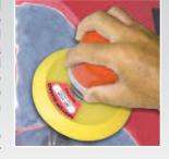
contact on irregular surfaces. Other accessories include a stiff, reinforced composite Backing Plate for aggressive sanding and grinding. Completing the line is a versatile Buffing Pad Holder for both lambswool bonnets and foam polishing pads. A hook facing provides a slip-free hold while allowing for quick change of pads.
