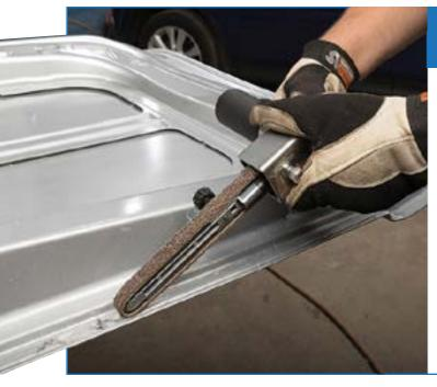
Remove spot welds faster than bits
