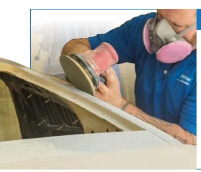
Aluminum oxide grain Strong paper backing Anti-loading
