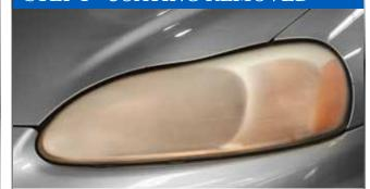
The lens can be wet sanded or dry sanded by hand with a sanding block or with a dual-action sander.
