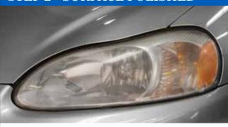
Scratch refinement can be accomplished by progressive sanding followed by a Lens Drier application to achieve a finish optimal for sealant.
