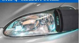
Use natural sunlight or the Presta UV Curing Light to cure the sealant on the restored lens. Headlight lenses properly restored with ReNuLite will last 1 year or more with the wipe-on application.
