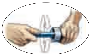
2 Chamfer & mark pipe
