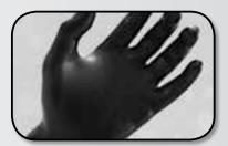
**Nitrile:** Nitrile is a synthetic polymer that has many natural rubber latex characteristics. Nitrile gloves are free of any latex proteins. Nitrile gloves provide better chemical and biohazard protection compared to latex gloves. Also, nitrile gloves are more resistant to punctures and tears compared to natural latex. Being a synthetic material, nitrile has a longer shelf life than natural rubber.
