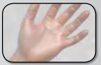
Vinyl: Vinyl is composed of a synthetic nonbiodegradable, protein-free material that includes polyvinyl chloride and plasticizers. Vinyl gloves are best used as an economical option for handling non-hazardous materials and chemicals.
