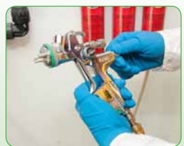
3 Assembly of the air cap - air cap marking must be legible
