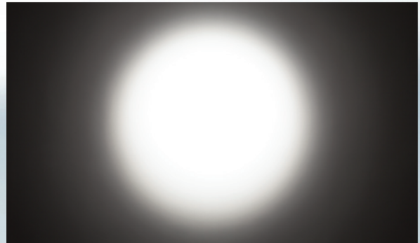
Light cone of the SATA® trueSun™ at maximum light power, uniform distribution of the light intensity edge to edge – color temperature is neutral
