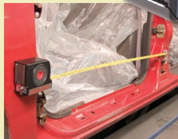
Four powerful magnets on side, back and bottom for hands-free measuring.
