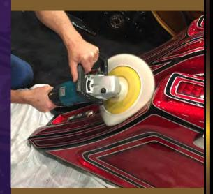
HINT: Your pad and product choice will determine the speed of cut and degree of gloss without fine pad scratches. Remember, wool cuts faster while foam finishes better. High density foam cuts more and the softer foam finishes best.
