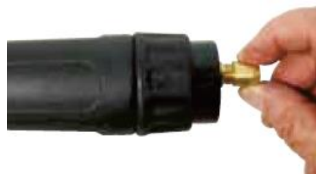
(2) Remove the liner retaining nut on euro end..
