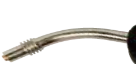
(1) Remove nozzle, tip, tip holder & diffuser.
