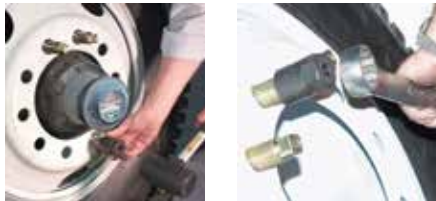
Special self-tapping splines
