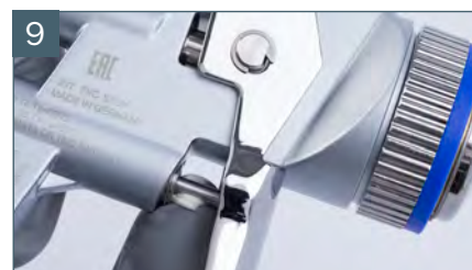
Grease visible part of air piston rod
