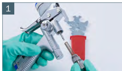
First remove paint needle.
