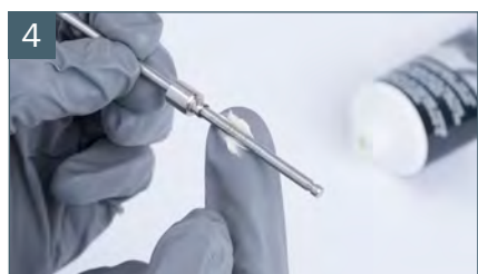
Grease paint needle around the needle packing area
