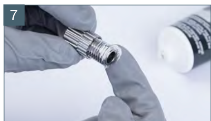
Grease thread of material flow control screw
